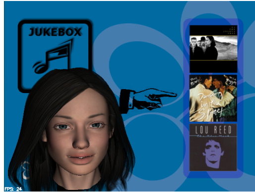
Figure 1.8: Example of proposed Talking head interface for MP3 player. The head is navigating the user through his/her music album collection. Examples of some ECA's gestures (head movement, background picture, pointing on the screen)
